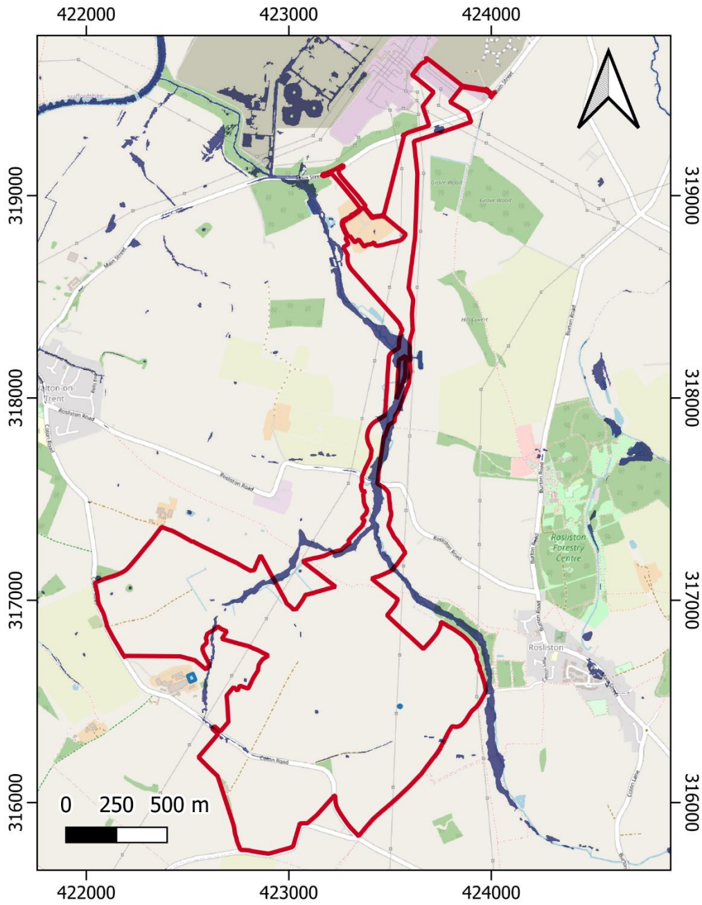
Figure 4-2 Flood risk from surface water
